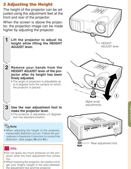
Hold the projector firmly while lifting or carrying.
